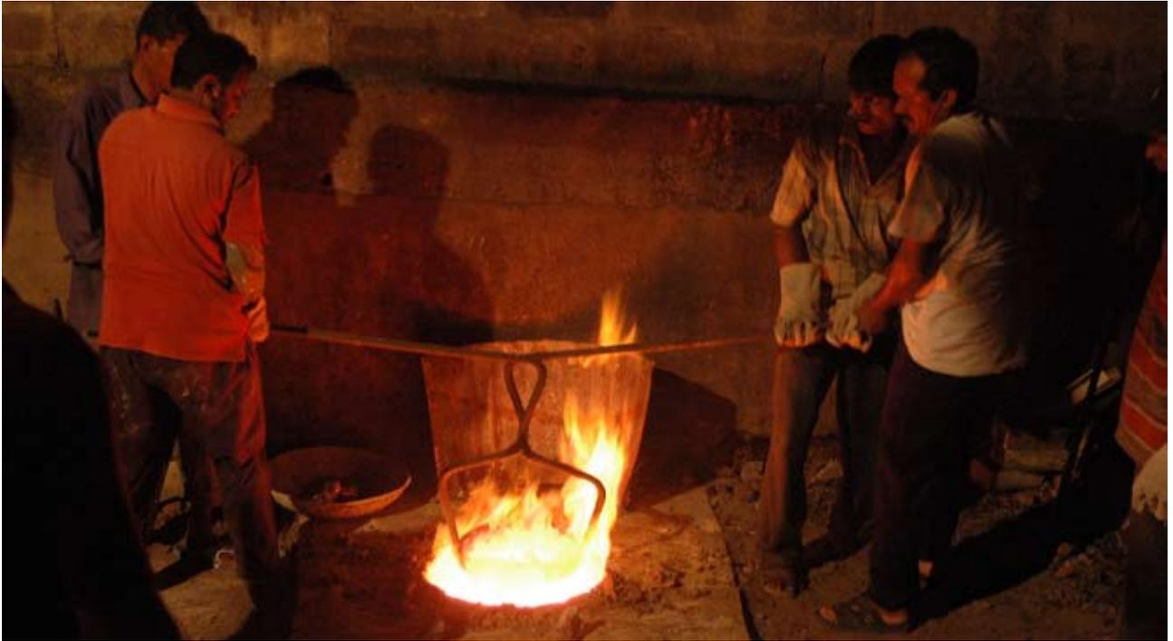
to assure even and thorough filling with liquid metal. In order to avoid air pockets, vents have to be attached carefully at the right places, as well as canals and conduits to facilitate distribution and easy flow of metal. All this shows, after the removal of the clay, as a treelike network of metal branches, which, when invisible in the hollow inside of the statue, add to its structural firmness, but are very disturbing when visible on the outside.
